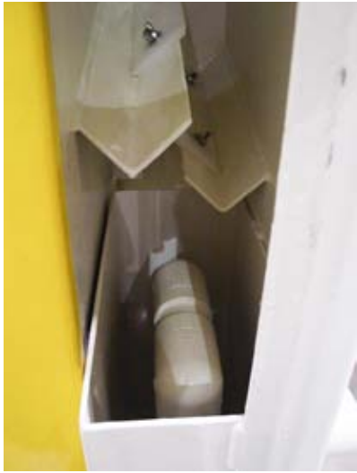
Self-adjusting wipers and oil removal from both sides of belt.
