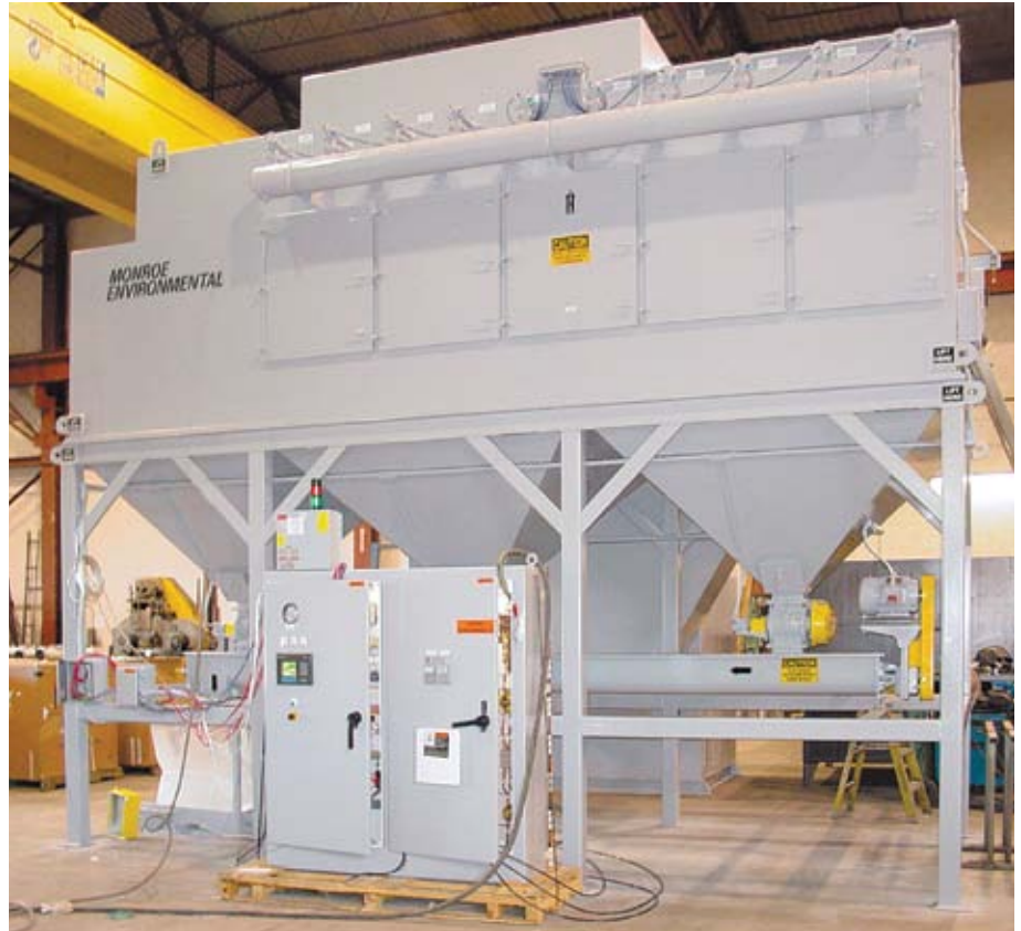
Custom configurations, including ceiling or roof designs, are available where a standard collector cannot be used. 30,000 CFM Dust Collector with screw auger option for dust removal shown.
